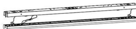
2. Untie the steel wire safety rope, Then untie the male female plug-in terminal and terminal
