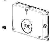
6. Remove one of the G1/2-14threaded plug at one side of the fixture.
