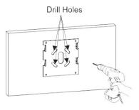
Drill holes with percussion drill in line with the hole position from wall
