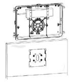
6. Install the lamp base on the wall mounting bracket
