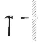
5. Use a hammer to drive the nylon expansion tube into the drilled hole on the wall.
