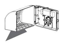
Power-on and testing to check if the luminaire works normally, screw up at last if no problems. (Note: Keep the waterproof silicone ring at the original position.)
