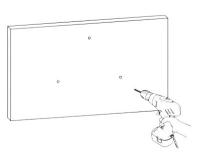
4. Drill holes on the wall according to the three screw holes of the bottom housing.
