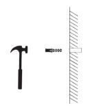
2. Use a hammer to drive the nylon expansion tube into the drilled hole on the wall.
