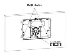
3. Fit and adjust the bottom cover at the right position according to the gradienter on the fixture.
