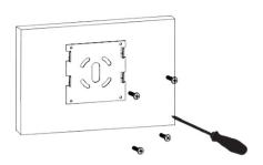
3. Fix the bottom housing on the wall with a self-tapping screw.
