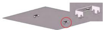
Fasten the clips to the mounting surface with the expansion screw. The distance between the clips: 382mm-0.6m; 982mm-1.2m; 1282mm-1.5m
