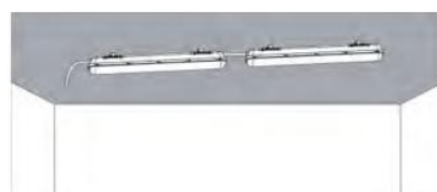
Fasten the mounting clips to the ceiling with expansion screw, then connect the lights with a cable and fix the lights to the clips
