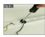
Step 6: Take out the LED driver and screws we provide; fix the driver onto the position of the previous ballast.
